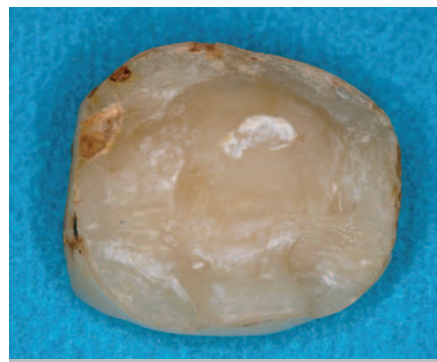
Figure 1 View of the intaglio surface of a displaced laboratory-processed composite onlay that de-bonded 8 years after placement with a 3-step total-etch system and dual-cure luting resin. I have seen this sometimes happen, over time, with all classes of dentin bonding agents.
